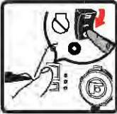
3. Turn the fuel selector switch to "LPG" position (1:30 o'clock). The gasoline valve is close on this position.
