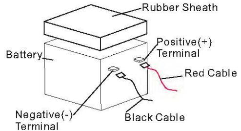
5. Pull out the battery and replace with new battery: 12V sealed lead acid 5.5AH LXWXH:90X70X100mm(3.54X2.76X3.84in)
