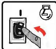
8. Push the battery power restore switch for about 3 seconds and then release.
