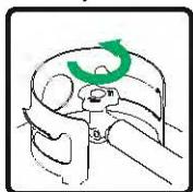
5. Turn the fuel selector switch to "LPG" position(1:30 o'clock).
