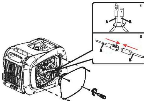
3. Insert the male connector of cable **A** into female connector of cable **B**.
