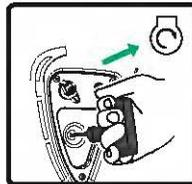
10. Push the choke button to the "RUN" position.
