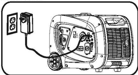
There is a light on the charger. This light will remain red until the battery get charged and then it will be changed to green. The charger won't charge the battery or will stop charging when the light is green to prevent any damage to battery and generator.
