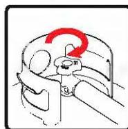
4. Turn the fuel selector switch to **"GAS"** position (4:30 o'clock).
