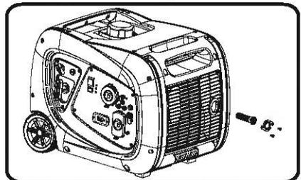
3. Carefully remove the carbon deposits from the spark arrester screen with a wire brush.
