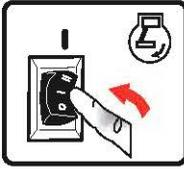
7. Push the battery power restore switch for about 3 seconds and then release.
