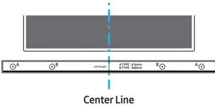
3. Push a pen tip or sharpened pencil tip through the center of the **A-TYPE** images on each end of the Guide to mark the holes for the supporting screws, and then remove the **Wall Mount Guide**.
