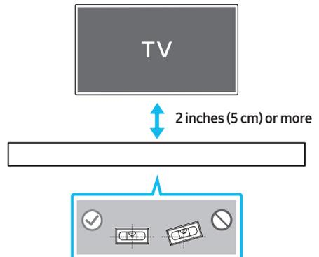
2. Align the **Wall Mount Guide's Center Line** with the center of your TV (if you are mounting the Soundbar below your TV), and then fix the **Wall Mount Guide** to the wall using tape.
