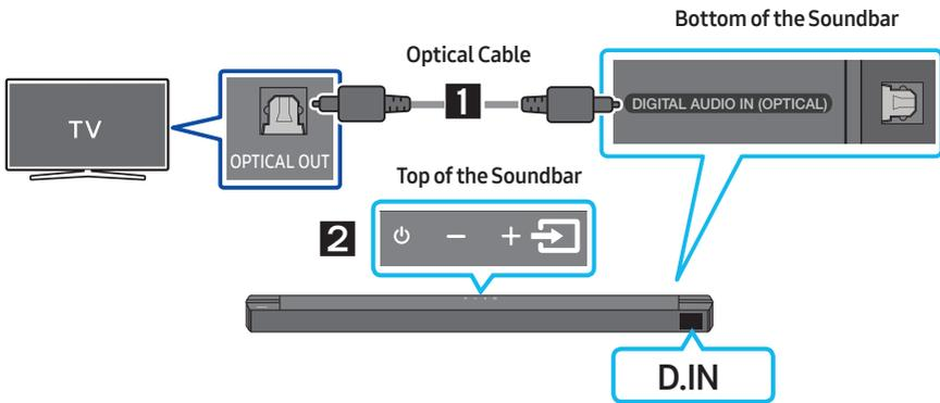
1. Connect the **DIGITAL AUDIO IN (OPTICAL)** port on the Soundbar to the OPTICAL OUT port of the TV with a digital optical cable.
