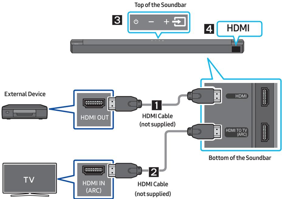
1. Connect an HDMI cable (not supplied) from the **HDMI** port on the bottom of the Soundbar to the HDMI OUT port on your digital device.
