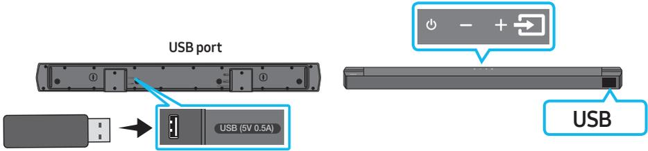
1. Connect the USB device to the USB port on the bottom of the product.
