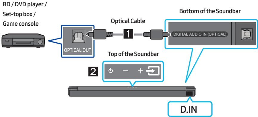
1. Connect **DIGITAL AUDIO IN (OPTICAL)** on the main unit to the OPTICAL OUT port of the Source Device using a digital optical cable.
