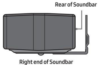
7. Install the Soundbar with the attached **Bracket-Wall Mounts** by hanging the **Bracket-Wall Mounts** on the **Holder-Screws** on the wall.
